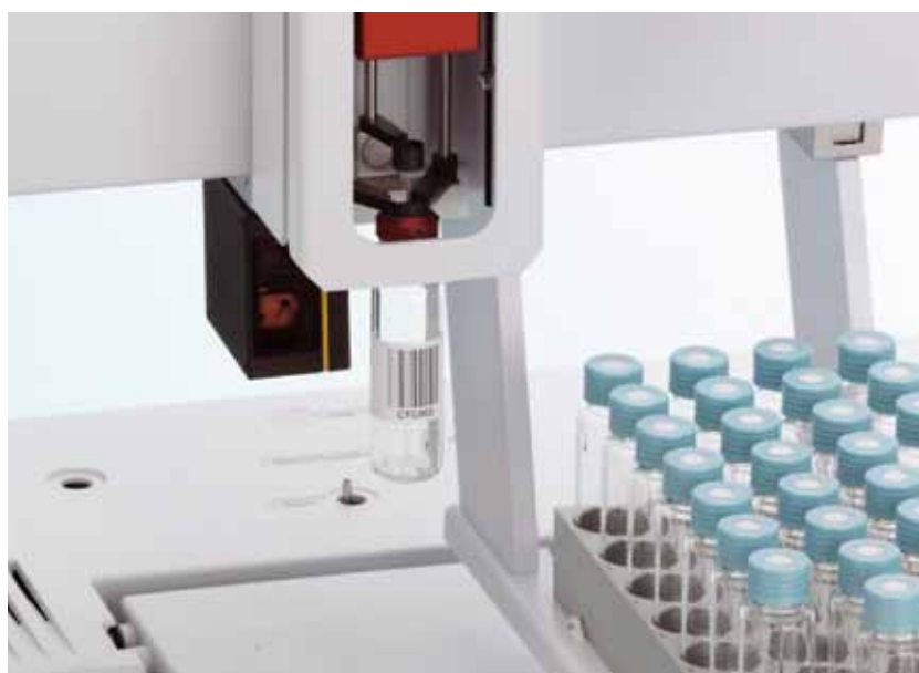
PAL COMBI-xt equipped with Barcode Reader
